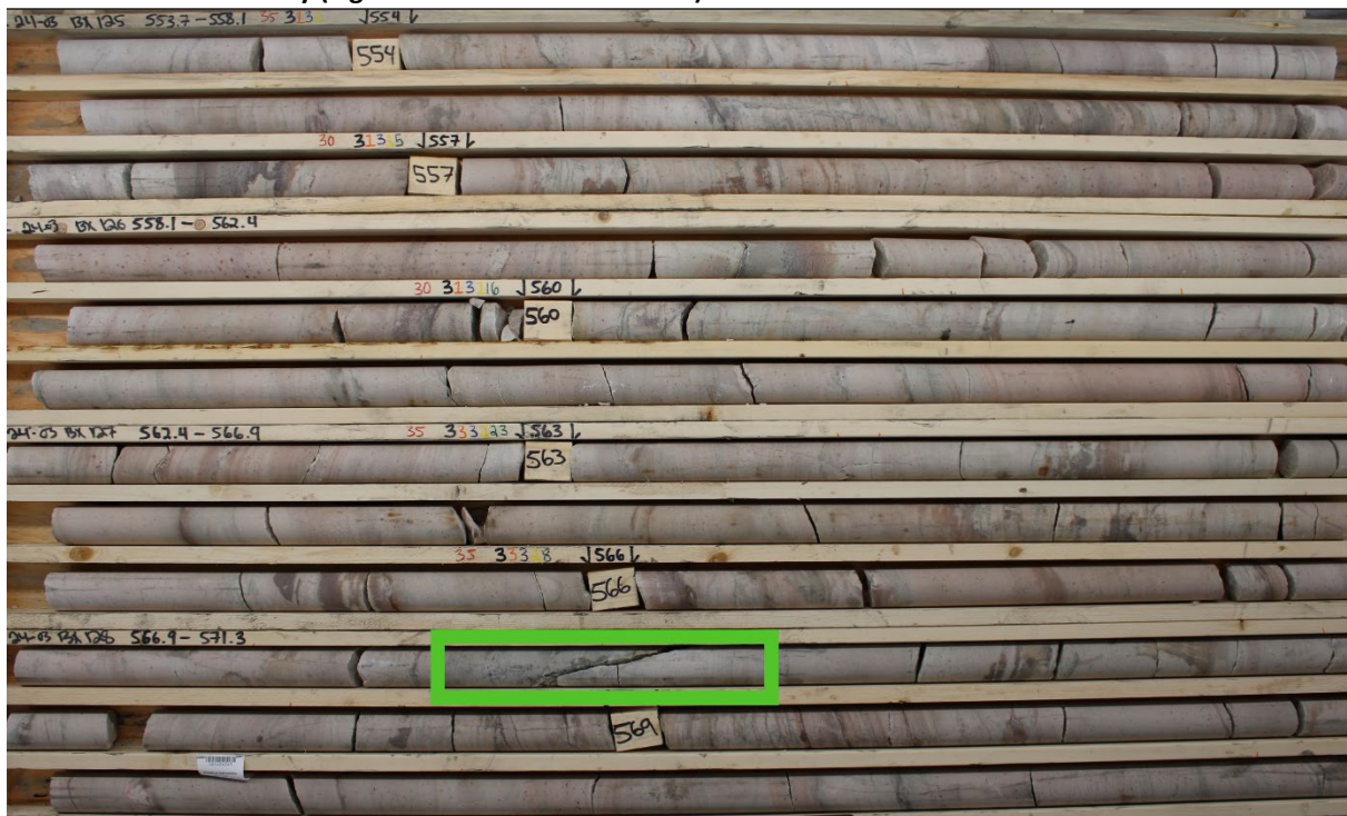
Figure 5 – Pervasively Bleached Sandstone from UR24-03 (553.7 – 571.3 metres) 450 metres above the sub-Athabasca Unconformity (Figure 6 Area Shown in Green)
