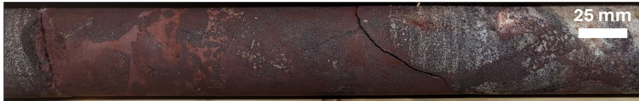
Figure 8 - Dravitic Breccia with Hydrothermal Hematite, Magnetite, and Pyrite from UR24-03 (752.3 m)
