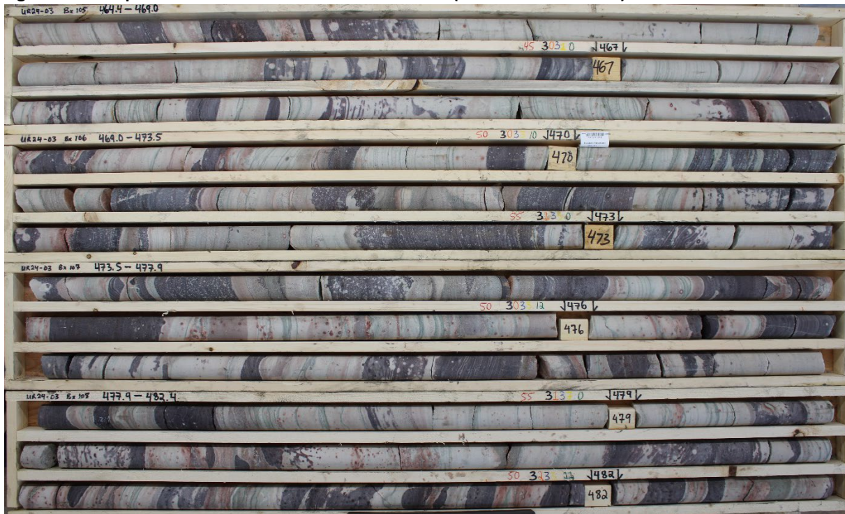
Figure 5 – Pervasively Bleached Sandstone from UR24-03 (553.7 – 571.3 metres) 450 metres above the sub-Athabasca Unconformity (Figure 6 Area Shown in Green)
